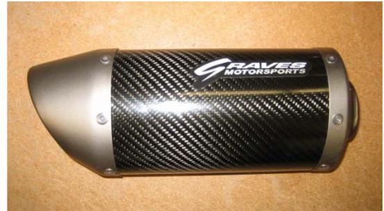
*For hassle free optimal performance there are complete replacement silencers for most **GRAVES** exhaust systems.*
