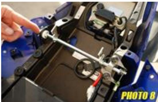
10. Remove the plastic fastener on the tool kit tray (photo 9)
