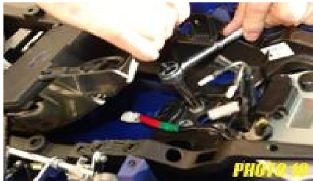
12. Install the fender eliminator bracket using the stock bolts and supplied nuts.
