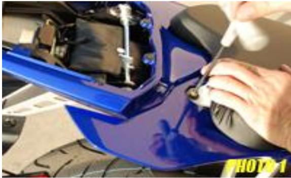
2. Remove the body panel under the passenger seat by removing the 4mm allen bolt and removing the 6 plastic snap fasteners (**photo 2**). Use a punch to push the center of the plastic snap fasteners.
