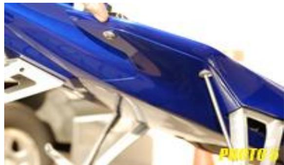
6. Remove the four plastic #2 phillips fasteners (**photo 6**). Remove the body panel.
