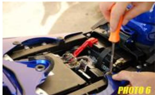
7. Remove the four 4mm allen seat mount bolts and the four #2 phillips head screws. (photo 7)
