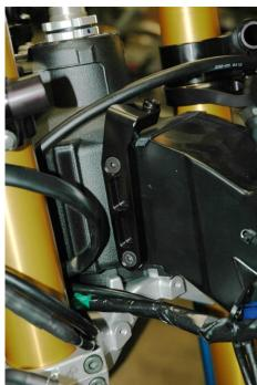
Once the key switch is removed install the top bridge bracket in its place using the supplied 8x25mm hex flanged bolt. Apply thread locking compound and torque to 30 Nm / 22 ft.lbs. 4) Install steering damper (see photo) using the supplied 8x30mm bolts and spacer. Apply thread locking compound and the pinch bolt torque (15 Nm / 11 ft lbs).
