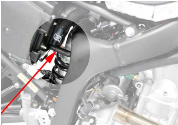
Photo 2 - Install rubber plug onto airbox.
