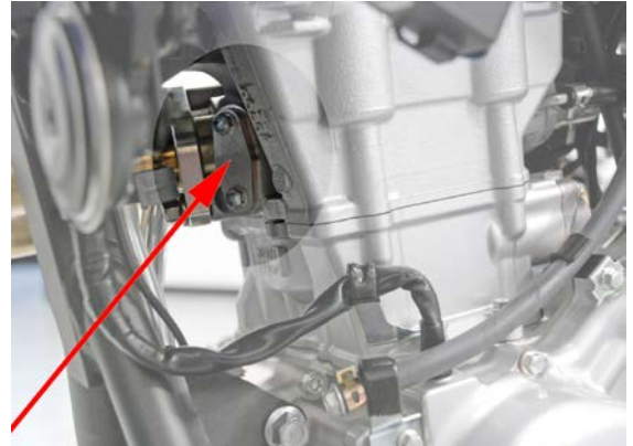
Photo 3 - Install block-off plate onto cylinder head.
