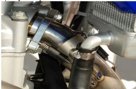
PHOTO 3 - head pipe spring installation
