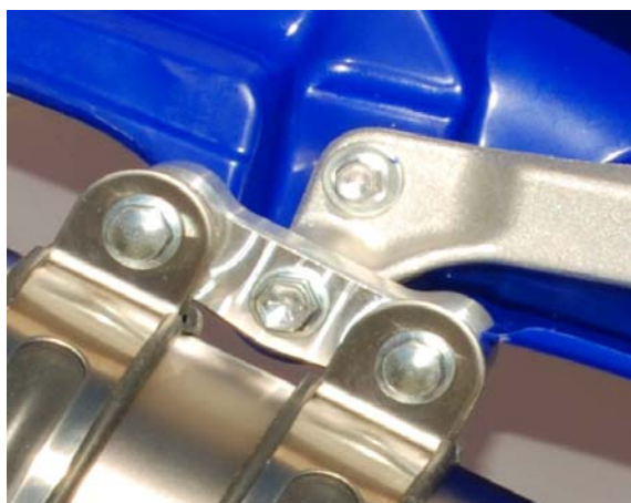
PHOTO 1– mounting bracket and hanger strap installation
