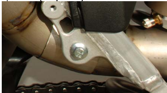
PHOTO 2 – mid pipe bolt installation
